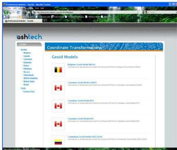
After a new geoid has been downloaded to your computer, run the downloaded “install.exe” file to install the new geoid on your computer (for use in your office software), and your receiver (for use in your field software) if it is currently connected to the computer via ActiveSync and the docking station.
